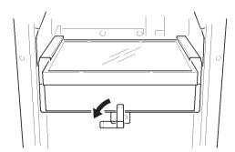
3 Pull out the light source carefully along the guide while holding it with both hands.
