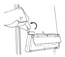
5 Holding the latch with one hand, remove the Epi light by pulling it gently outwards.
