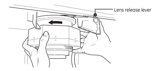
8 Rotate the lens to the left by 45 degrees.
