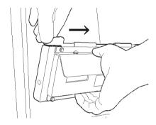
10 Lower the latch to lock the Epi light in place.
