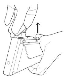
7 Before installing the new Epi light, ensure that the latch is sprung open (upwards).
