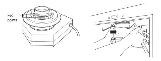
6 Raise the lens into position and rotate it clockwise to lock in position.
