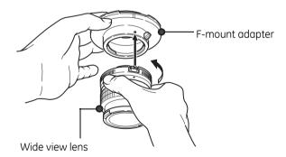
7 Fix the lens in position be turning it to the right.
