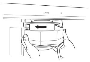
**Note:** Hold the lens with both hands so as to prevent the lens guide from being damaged.
