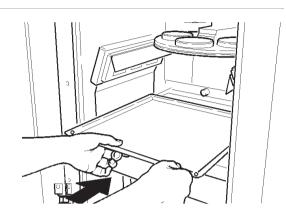
5 Ensure the lens cap is removed and close the IDX door.
